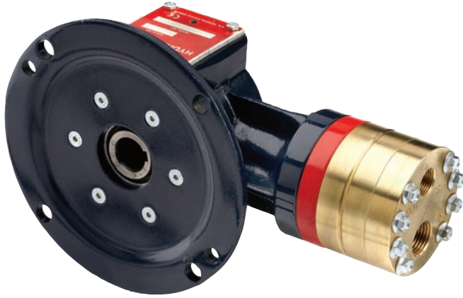
F20/G20 close-coupled for 56C frame or IEC 80 footed motors shown. G22 models to IEC 80 - 90 B5 frame motors. Pump head materials include (metallic) Brass, 316L Stainless Steel and Hastelloy C and (non-metallic) Polypropylene and PVDF.
