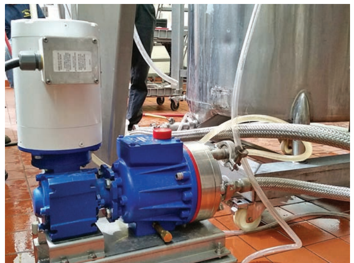
P400 used for spray drying of non-lubricating as well as viscous flavor additives in the food processing industry.
