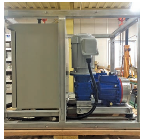
Ground stabilization in an earthquake zone requires precise metering, a small footprint, and virtually pulse-free flow provided by this P400.
