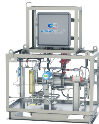
IntellijECT PLC controlled fully automated portable 8400 high pressure injection package with local, remote and automated flow control with flow, pressure and temperature transmitters, actuated discharge ball valve and fire fuse for emergency shutdown. Class 1, Div 1. Final destination: GOM
