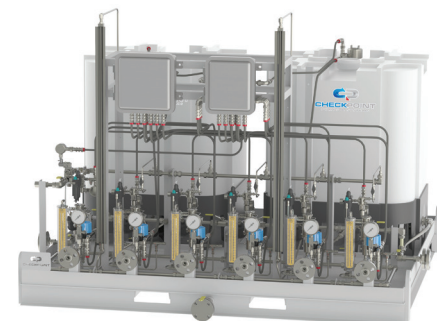
Six pump 1250 injection package with two 275 gallon poly tote tanks with level transmitters, flow switches and emergency shutdown solenoid valves. Final destination: Bolivia
