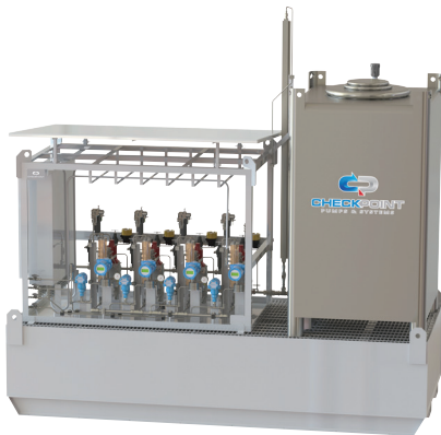
Quad pump pneumatic 1250 auto ready injection package remote and local flow control, solenoid valves for emergency shutdown, flow and pressure transmitters, and 550 gallon 316SS tank with level transmitter and 130% containment bund. Three primary pumps, one fully redundant backup (3A + 1B). Final destination: Marshall County, WV
