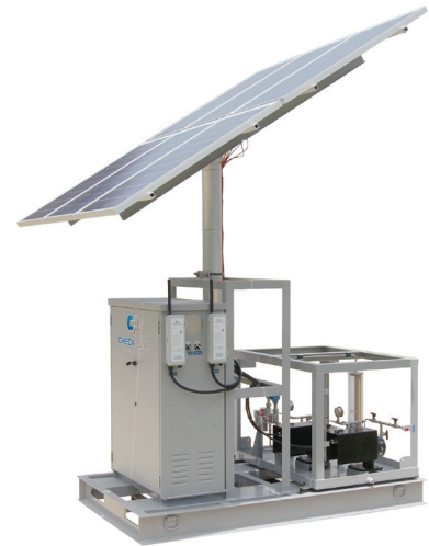
Solar powered dual FXS fully automated injection package with IntellijECT-Lite cellular communications for automated proportional chemical flow with tank level monitor and remote or local flow adjustment. Final destination: Permian Basin, TX
