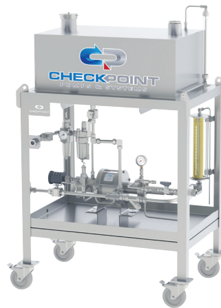
NACE compliant portable 6212 batch treatment injection package with 2507 tubing and fittings, custom fabricated top mounted 35 gallon SS316 chemical tote tank with level gauge and flame arrester. Final destination: GOM floating drill rig
