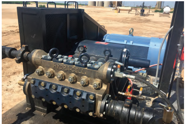
T and Q Series pumps feature the Hydra-Cell seal-less design, eliminating clean-up costs from leaking seals or packing and protecting operators from dangerous fluids such as those containing hydrogen sulfide (Q155 shown).
