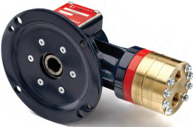
F20 Close-coupled for 56C frame motors shown. F21 models are shaft-driven. F22 models are flexible-coupled to 56C, 143TC and 145TC frame motors. Pump head materials include (metallic) Brass, 316L Stainless Steel and Hastelloy C and (non-metallic) Polypropylene and PVDF.
